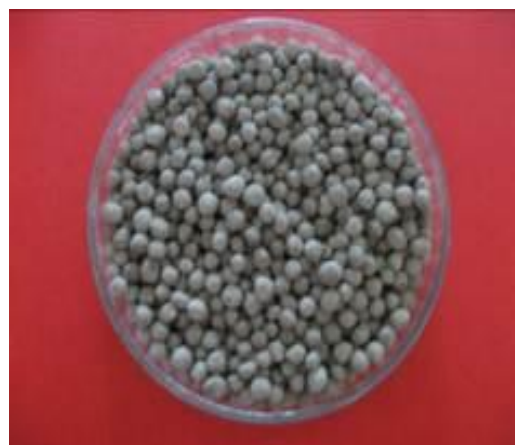
Figure 1. Bio-superphosphate in granular size of 2-4 mm in diameter.
